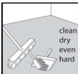
Podium 30, PRO 55, XXL and XXL XTRA are dry-back tiles and must be fully adhered to a smooth, hard, clean (free from dust and small particles) and permanently dry subfloor (incorporate a damp proof membrane where there is a solid subfloor.)
